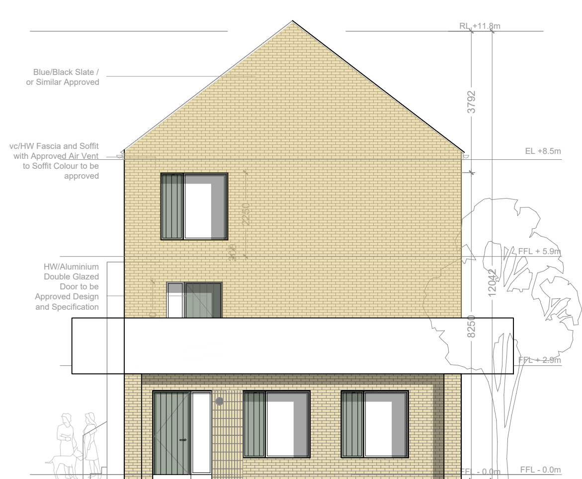
06 100 REAR ELEVATION 1:100 BLOCK-10-T1.1
